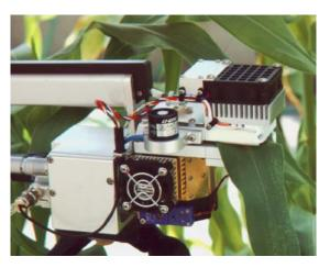
The 6400-02B is designed for easy field operation. Mounting is as simple as replacing the upper half of the standard leaf chamber with the light source. The 6400-02B is controlled by the LI-6400/6400XT software and powered by the system batteries, so there are no extra boxes, cables or power sources to carry.
